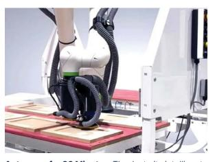
**Autonomy for 20 Minutes:** Thanks to its intelligent design, the PSA-80 PRO allows employees to focus on other tasks while it handles sanding autonomously.
