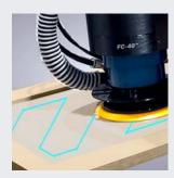
**Criss-cross pattern** optimizes sanding toolpath for MDF/HDF sanding.
